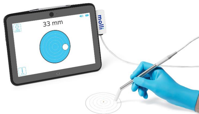
Figure 2: Oncopen detecting the marker with directional feedback showing on the screen of the MOLLI 2 tablet
